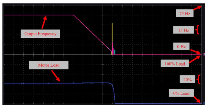
Figure 3: Output Frequency and Motor Load During Deceleration (25 seconds ramp down)
